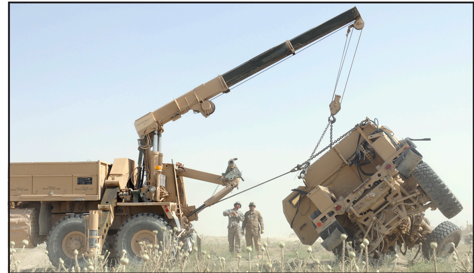
Spc. Larry Smith, a mechanic with the 131st Transportation Company, a Pennsylvania National Guard unit attached to the 101st Sustainment Brigade, and Sgt. 1st Class Alvin Beehler, the chief instructor for the vehicle recovery course from the 59th Ordnance Brigade, US Army Ordnance Center and School, flip a mine resistant ambush-protected vehicle with an M984 HEMTT wrecker. (U.S. Army photo by Spc. Michael Vanpool)
