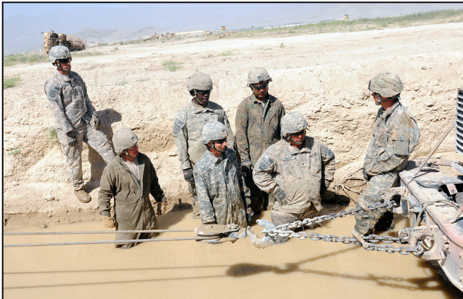
Sgt. Joshua Garner, a recovery instructor with the 59th Ordnance Brigade, US Army Ordnance Center and School, walks the six students of the Vehicle Recovery Course through different approaches to recovering a vehicle stuck in a mire pit. (U.S. Army photo by Spc. Michael Vanpool)
