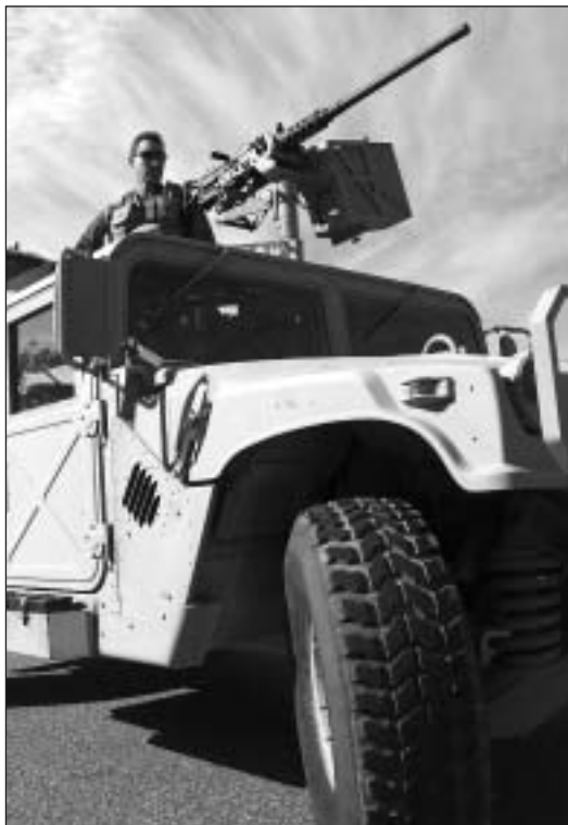
A soldier from the 3rd SF Group looks down the barrel of an M-2 .50-caliber machine gun mounted on a Ground Mobility Vehicle, or GMV. The GMV is in use by SF soldiers deployed in support of Operation Iraqi Freedom.
