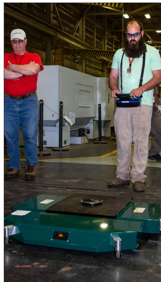
Production Machinery Mechanic Ethan Holland operates the TK-EVO Heavy Lifting Device using a remote-controlled device.
