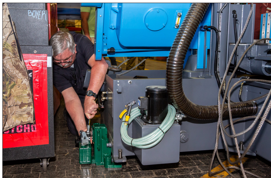
LEFT: Production Machinery Mechanic Ethan Holland operates the TK-EVO Heavy Lifting Device using a remote-controlled device. TOP: The TK-EVO Heavy Lifting Device and the remote-controlled device. BOTTOM: Mechanics set up the load onto the main crawler using the toe jacks.
