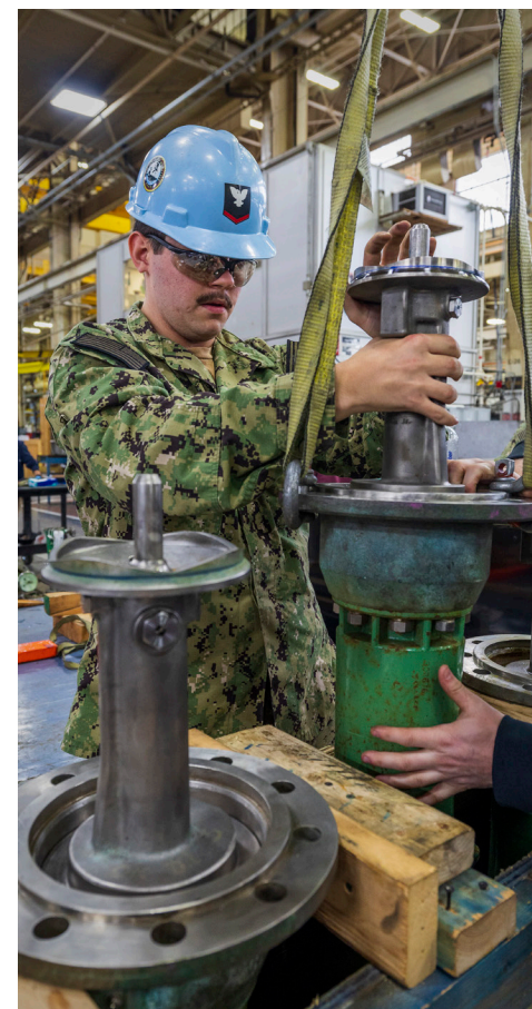
LEFT: Dylan Whaley, an electricians mate third class assigned to USS Theodore Roosevelt (CVN 71), assists with a valve repair in Shop 31, Machinists, Electroplaters & Toolmakers. Sailors were trained on repairs in a new collaboration between the shop and the ship. BELOW: Whaley, center, gets help disassembling a valve from Erik Kendrickson, right, a technician from contracting partner Curtiss Wright Fleet Solutions and John Devito, left, a technician from contracting partner Target Rock. (U.S. Navy photo by Wendy Hallmark)
