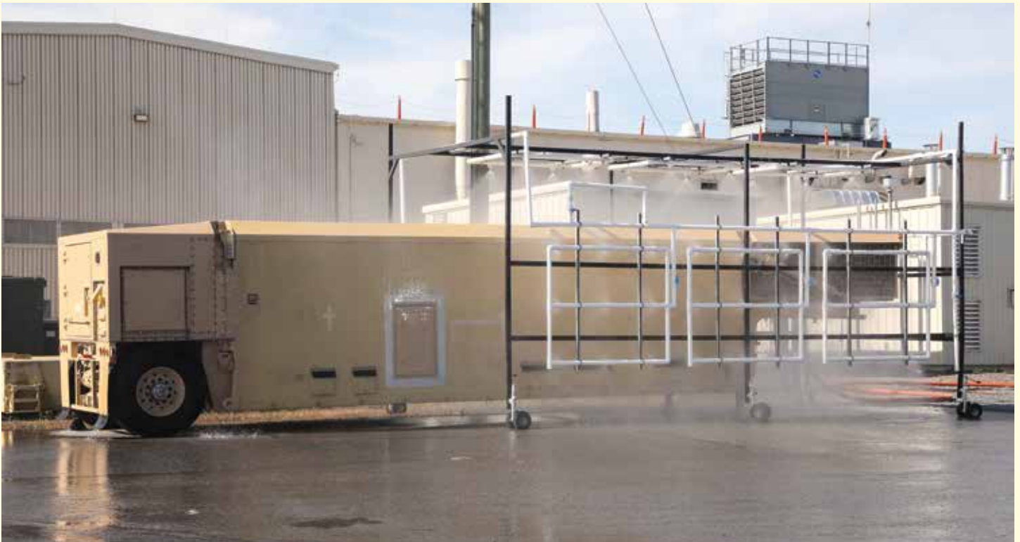
An AN/TPY-2 Electronics Equipment Unit undergoes rain testing at Letterkenny Army Depot Oct. 14, 2020. Letterkenny employees constructed the apparatus used to execute the test. (U.S. Army photo by Pam Goodhart)
