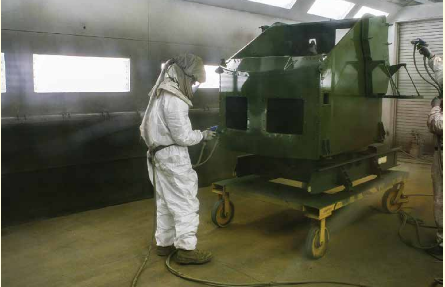
Painters in the Directorate of Industrial Operations at Letterkenny Army Depot apply paint on an Avenger turret Oct. 15, 2015. (U.S. Army photo by Pam Goodhart)
