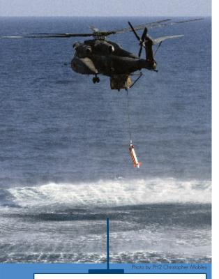
A MH-53E Sea Dragon assigned to the "Vanguard" of Helicopter Mine Countermeasures Squadron Fifteen (HM-15) retrieves an AN/AQS-14A Side-Looking Sonar used to detect underwater mines in it's support of Mine Warfare Readiness and Effectiveness Measuring (MIREM) Program 27 to collect and analyze mine warfare data. The data collected will be used to develop a database that can use to weigh decisions on proposed system improvements. HM-15 is a Navy Reserve squadron from Corpus Christi, Texas.
