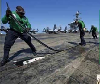
Sailors assigned to Air Department aboard the Nimitz-class aircraft carrier USS Carl Vinson (CVN 70) install slot seals on a catapult track after completing noload tests after a sandstorm swept across the flight deck. Photo by Mass Communication Specialist 2nd Class James R. Evans.
