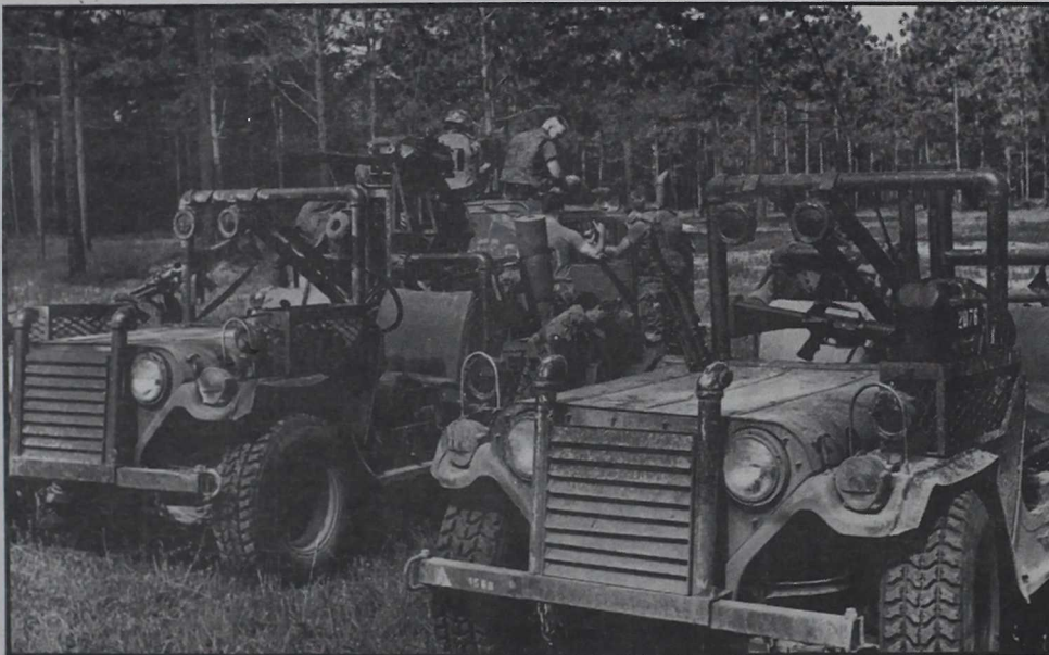
EASY TO SPOT —The Super Jeep's unique appearance makes it easy to identify even out in the field. Note the roll bars, two additional infrared lights, larger than normal tires and steel radiator guard that is just a part of the Super Jeep's unusual appearance.
