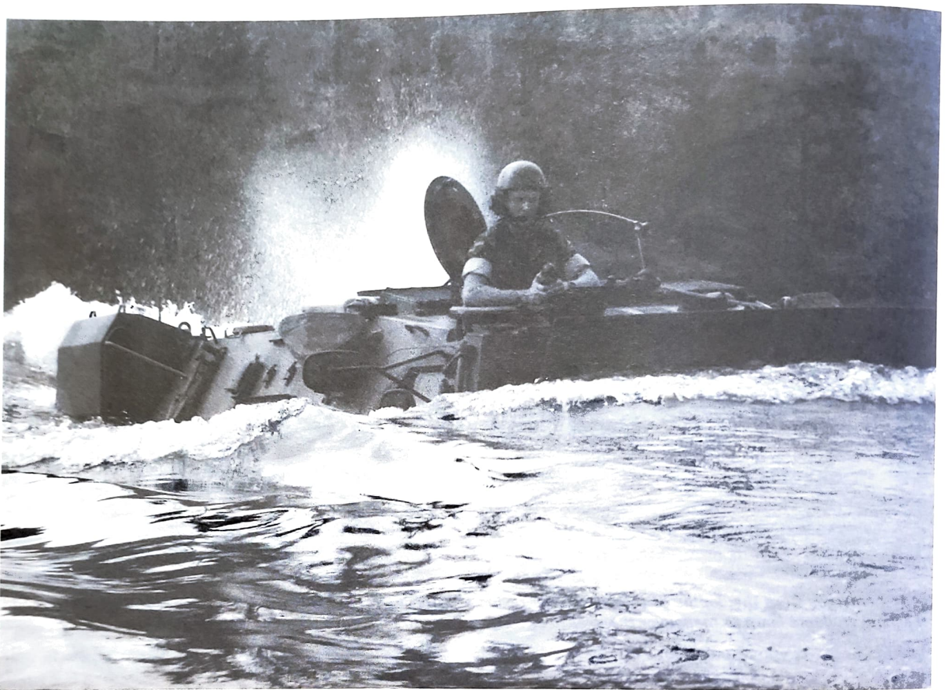
The Fox is an amphibious vehicle that can detect traces of nuclear, biological, and chemical agents. The six-wheeled transport carries a crew complement of four and is propeller-driven. It is a vital resource for chemical soldiers in ensuring the safety and well-being of troops, both on and off the battlefield.
