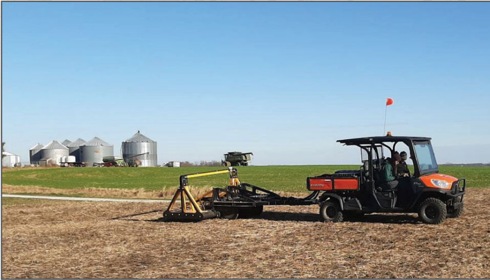
U.S. Army Corps of Engineers Louisville District Camp Breckinridge Environmental Restoration team uses the UltraTEM-IV technology to conduct a geophysical survey at Camp Breckinridge Military Munitions Response Program Project 06.
