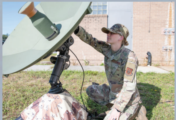
Senior Airman Kimberly Nelson, 919th Special Operations Communications Squadron radio frequency technician, checks the configuration of a data satellite at Duke Field, Florida, Oct. 14, 2021. The satellite can provide high speed data downloads for special operations missions and gives deployed commanders the ability to communicate around the globe. Photo by Michelle Gigante.
