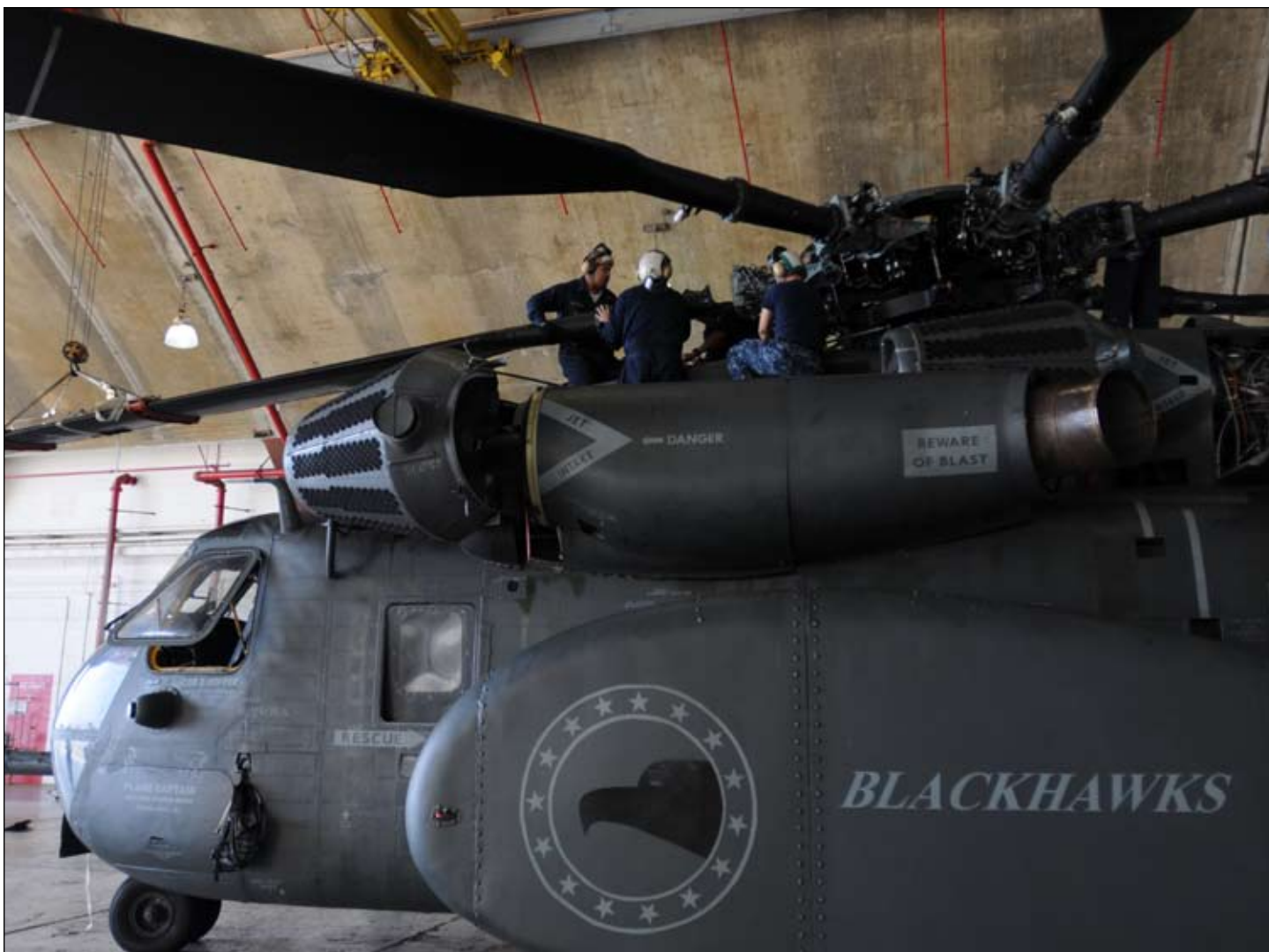
Crewmembers assigned to Helicopter Mine Squadron 15 (HM-15), attach a rotor blade to the rotor head of a MH-53E Sea Dragon at the U.S. Naval Station Guantanamo Bay airfield, Feb. 2, 2010. HM-15 is at Guantanamo Bay supporting Operation Unified Response following the 7.0 magnitude earthquake in Haiti on Jan. 12, 2010. – JTF Guantanamo photo by Navy Mass Communications Specialist 3 rd Class Joshua Nistas
