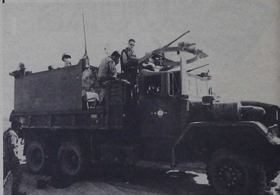
KING OF THE ROAD - A Force Logistic Command "War Wagon," a converted five-ton cargo truck, is readied for one of the daily convoy security runs conducted by Marines of the FLC's Truck Co. Armor plating, radio equipment, and a .50 caliber machinegun make the "War Wagon" a self-sustaining security vehicle for resupply convoys to support 1st Marine Division forces south of Da Nang. (Photo by LCpl. N.W. Myers)
