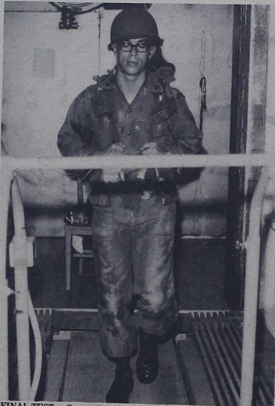
FINAL TEST — Corporal J.M. Molina, 2d Service Battalion, 2d Marine Division, nears completion of 30 minute treadmill walk in high temperature and humidity chamber. Wires leading from his waist monitor heart and metabolic rates.
