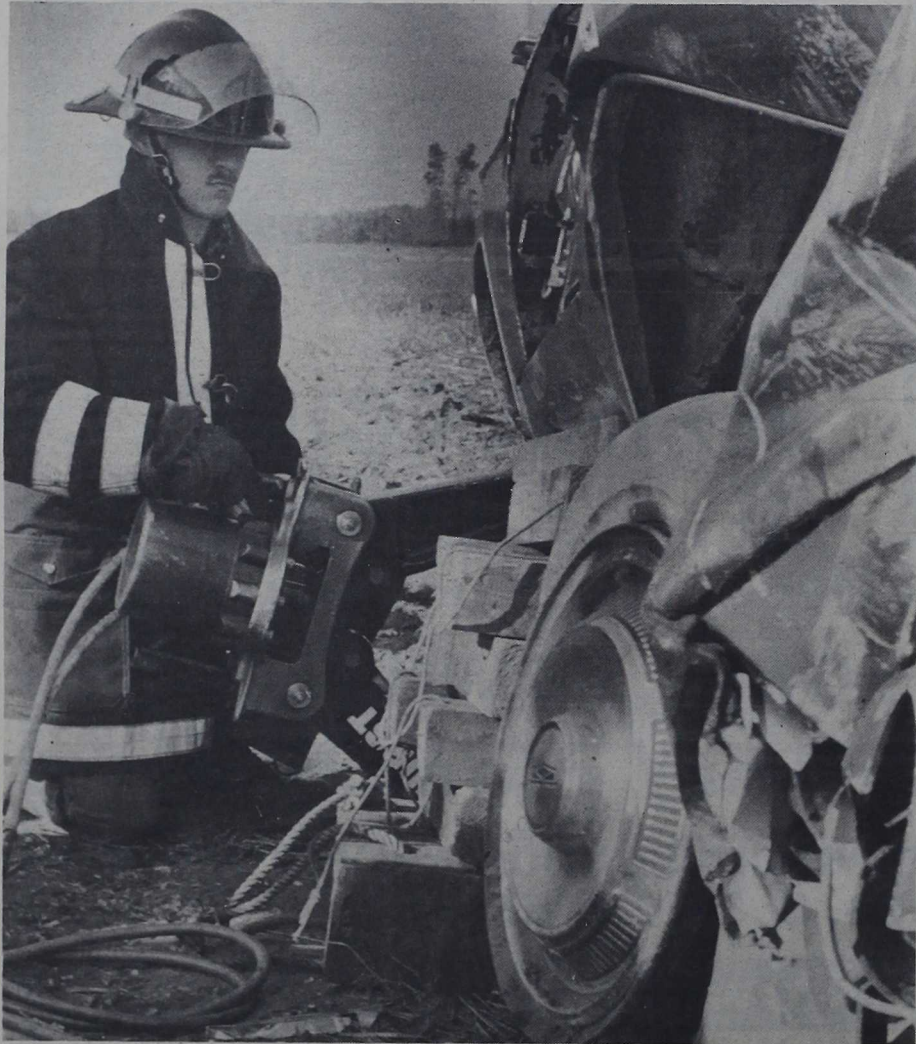
Petty Officer Third Class Scotty L. Pike, 3d Battalion, 8th Marine Regiment, uses the jaws of life to lift a car during training at an auto junkyard.
