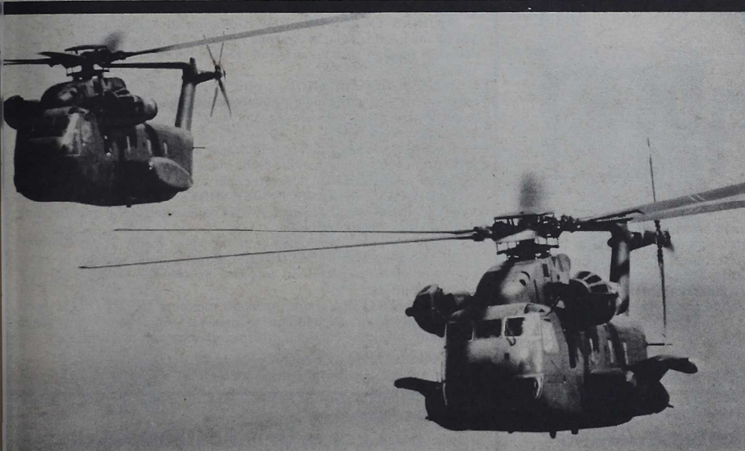
The heavy assault CH-53 Sea Stallion helicopter, designed specifically for the Marine Corps.
