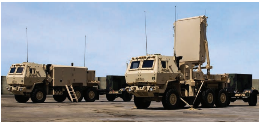
Figure 4. The AN/TPQ-53 is a C-130-transportable, truck-mounted counter-target-acquisition radar system configured to provide 360-degree threat-detection capability. It is able to locate the firing positions of both rocket and mortar launchers. the Q-53 requires a four- or five-man crew and includes a 60-kilowatt transportable generator and one support-shelter vehicle. Q-53 uses an encrypted wireless network able to reach up to 1,000 meters away. (U.S. Army photo by Kristen Kushiyama)
