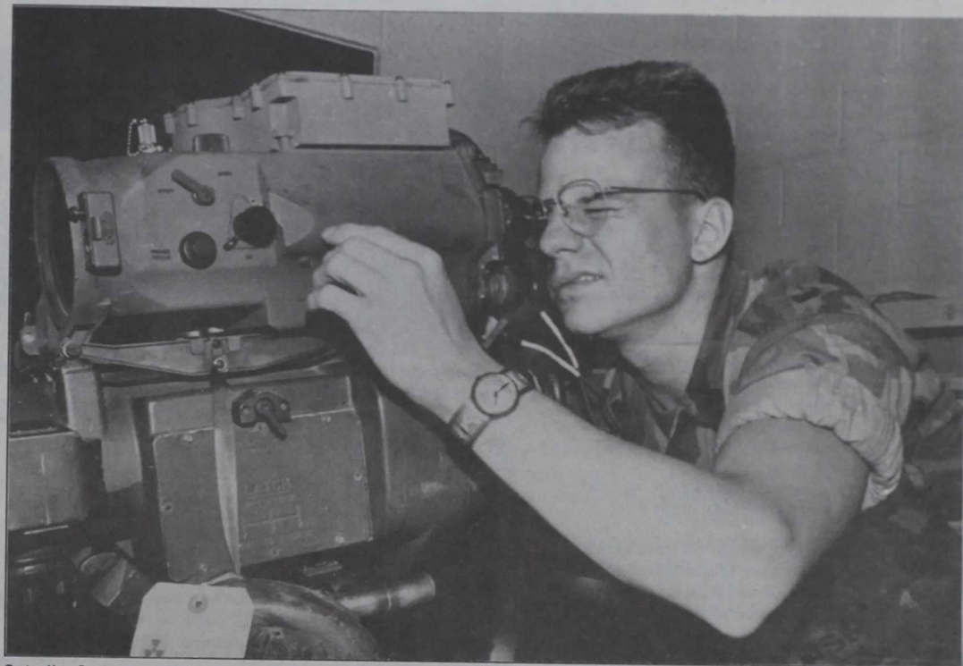
Sgt. Jim Scace, an optics repairman with Ordnance Maintenance Plt., fire control section, checks the sights on a TOW mount. The section fixes all of the sighting devices used by the Marine Corps.
