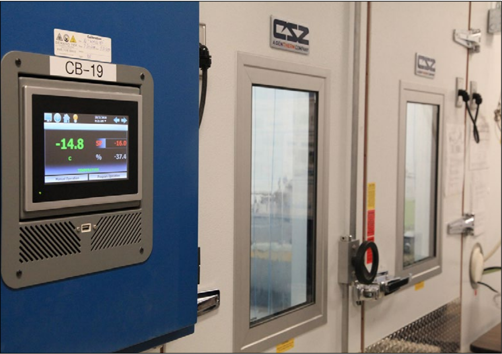
A photograph of the environmental chamber, or cold room, where ice growth and adhesion testing are conducted at temperatures from -8 °C to -20 °C. The chamber can reach -40 °C, which is important for studies with saline ices.
