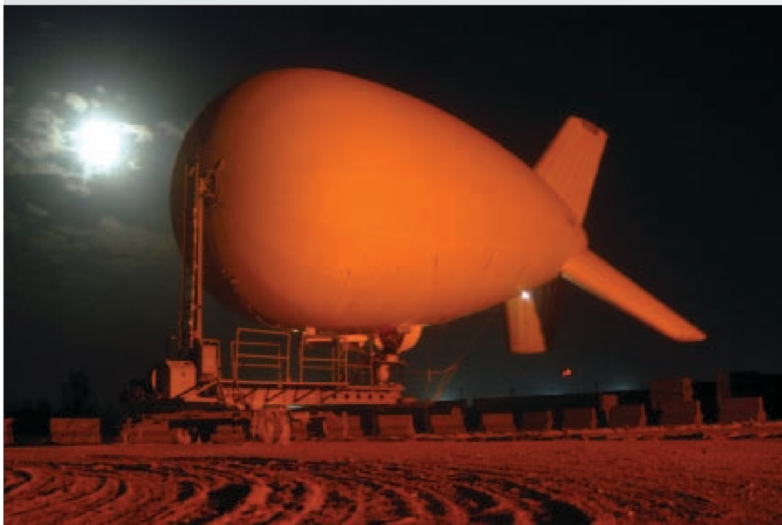
The 17-meter Aerostat of Contingency Operating Location Q-West secured to its mobile mooring station during a windy night Nov. 2. The aerostat — maintained and operated by crewmembers from A Company, 2nd Battalion, 198th Combined Arms, out of Hernando, Miss., and attached to the Base Defense Operations Center — provides a key element of base defense.
