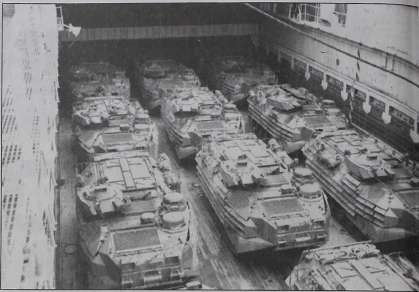
Amphibious Assault Vehicles (AAV's), mounted with a turret housing a 40mm grenade launcher and gun and capable of transporting a squad of Marines, line the well deck of the USS Portland, ready to be shipped to the coast during Non-combatant Evacuation Operations.
