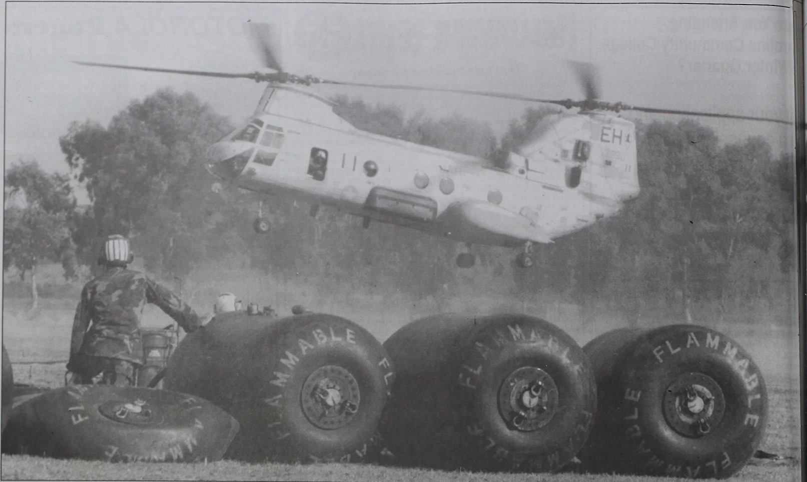
A CH-46 Sea Knight from HMM 264 comes into the Forward Arming and Refueling Point to get some gas. The 3,000 pound fuel bladders in the foreground will help keep other 'helos' in flight. GySgt. Tim Shear
