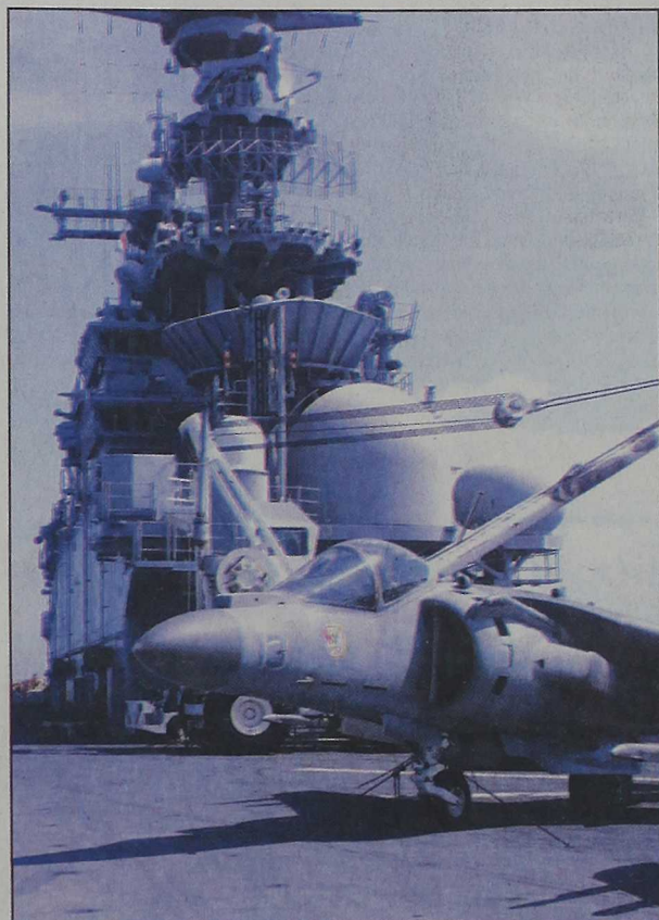
An AV-8B Harrier is secured to the USS Wasp flight deck. The ship is specifically designed to accommodate the jet, along with a full range of Navy and Marine Corps helicopters.
