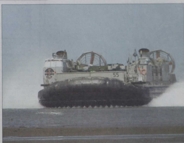
Marines and Sailors rush to shore on a Landing Craft Air Cushioned vehicle during a personnel and aircraft recovery exercise recently. The LCAC is a high-speed, over-the-beach fully amphibious landing craft capable of carrying a 60-75 ton payload. It is used to transport weapons systems, equipment, cargo and personnel from ship to shore and across the beach. Their payload and speed mean more forces reach the shore in a shorter time, with shorter intervals between trips.
