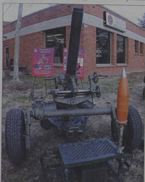
The Expeditionary Fire Support System is a mortar-based system designed to provide mobile fire support for expeditionary forces. The system utilizes a 120 mm rifled towed mortar that can fire rifled or smoothbore ammunition.
