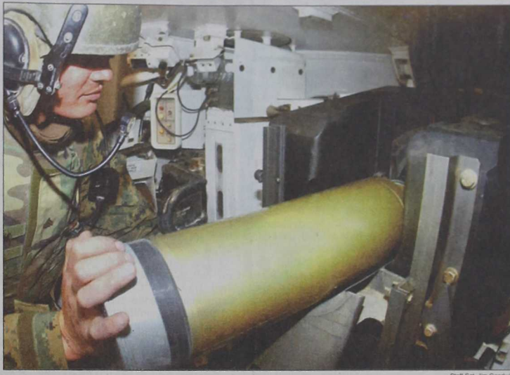
Corporal Lester P Brock, a 30-year-old from Brainard, Minn., and Marine tank gunner, loads a round into the 120mm main gun on an M1A1 Abrams Main battle tank during a live-fire training mission in the western desert of An Najaf Province, Iraq, Jan. 24.
