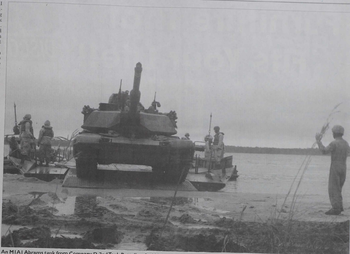
An M1A1 Abrams tank from Company D, 2nd Tank Battalion, 2nd Marine Division leaves a raft from Bridge Company, 8th Engineer Support Battalion, 2nd Marine Logistics Group after reaching the beach at Camp Devil Dog Oct. 10. Ten tanks and one M88 tank recovery vehicle were moved across the New River during a river-crossing exercise conducted to transport the heavy equipment in the most efficient manner. Photo by Staff Sgt. Juan Vara
