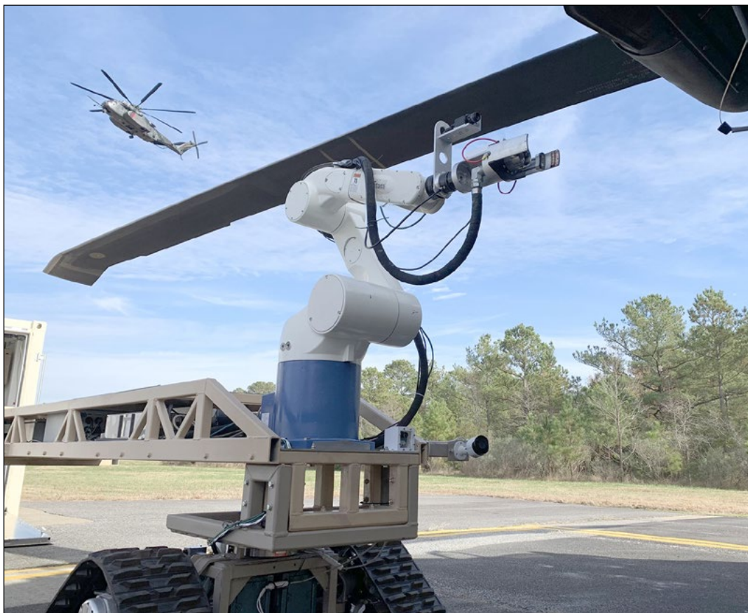
The Autonomous and Robotic Remote Refueling Point (AR3P) ruggedized system delivers fuel as a ground-based autonomous unmanned robotic arm refueling capability system that is rail mounted and deployed from a standardized shipping container. (U.S. Army Photo)
