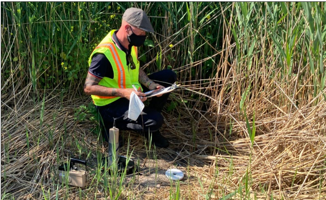
Shawn Andrews, health physicist, USACE Buffalo District, logs in the time of placement for a radon flux canister at the Tonawanda Landfill Vicinity Property. (Photo by Lisa Berta)
