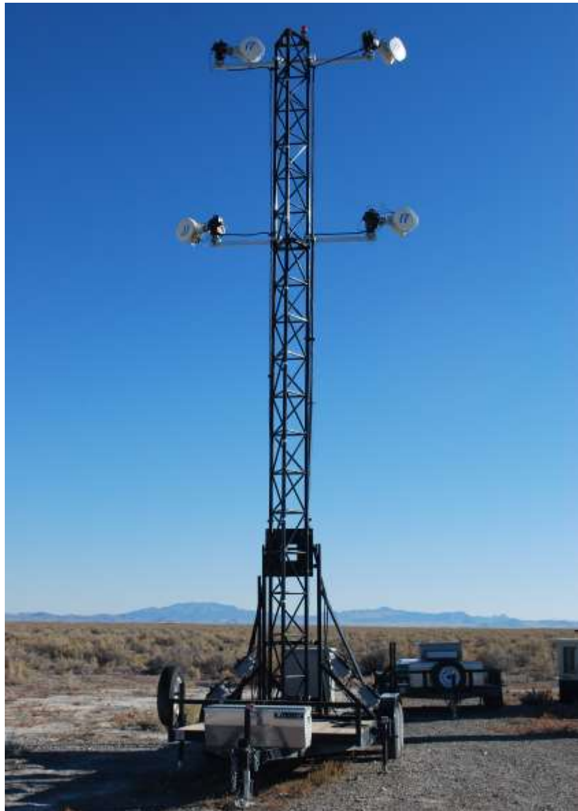
A trailer-mounted instrument tower used for outdoor testing of defenses against simulated chemical and biological agents at Dugway Proving Ground. The 10-meter tower folds down for ease in attaching instruments. The upgrade of hardware and software through OADMS depends upon this kind of mobility for test setup and, in the future, "safari" capability to take the testing system off DPG to other installations. Photo by Joe Mashinski
