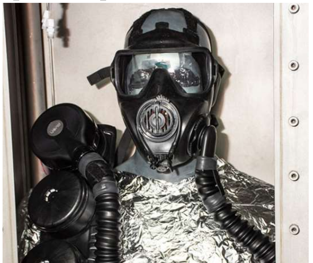
Lab testing of the M53 protective mask, a variant of the current issue M50, is completed. Testing determined whether the mask was degraded by exposure to Joint General Purpose Decontaminant for Hardened Military Equipment (JGPD-HME), created to decontaminate vehicles, ship surfaces and weapons exposed to chemical or biological agents.
