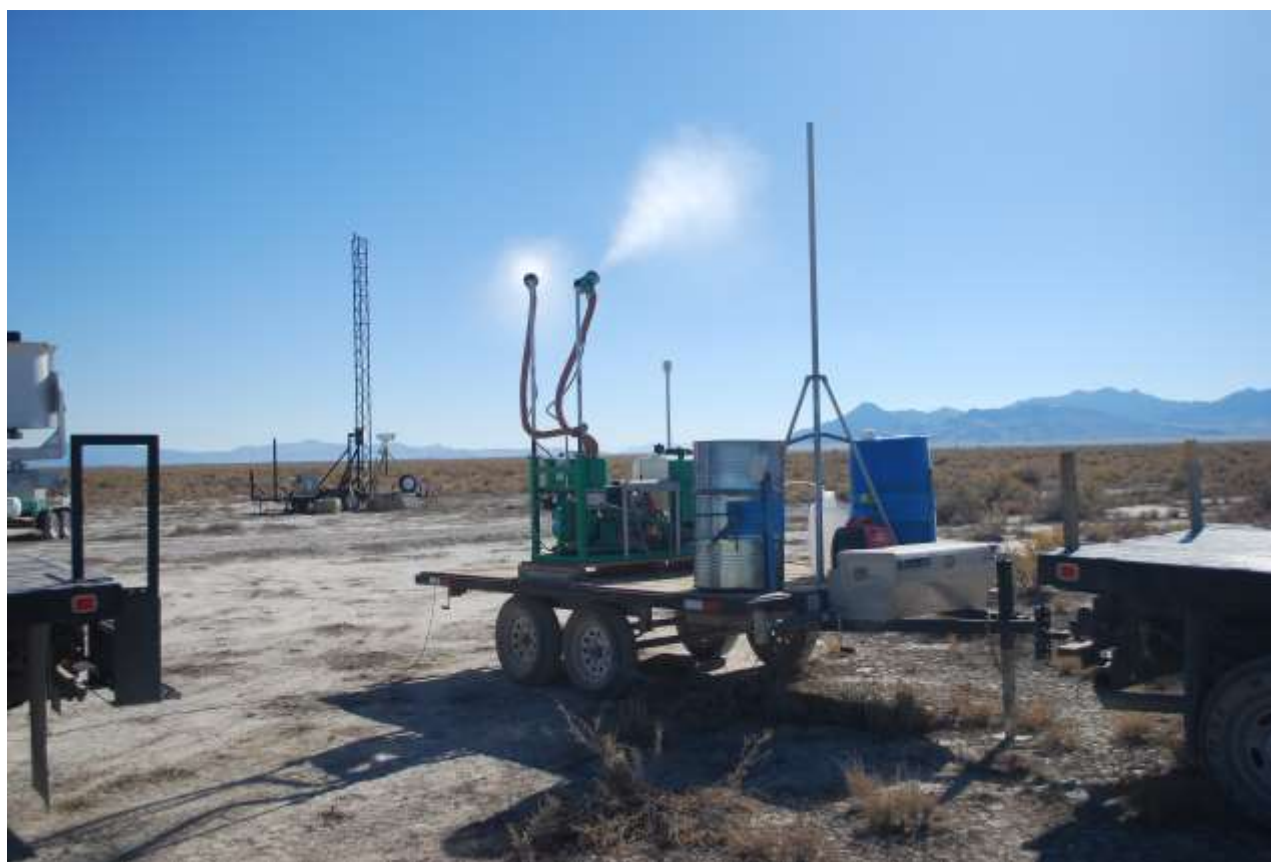
The OADMS upgrade will simplify the collection of data after a disseminator, shown here, releases simulated chemical or biological agent to challenge a detector. Decades-old international agreements ban the release of actual chemical or biological agents outdoors, so simulants are used. Testing with actual agents is done in sealed chambers with multiple levels of containment and filtration. Photo by Joe Mashinski
