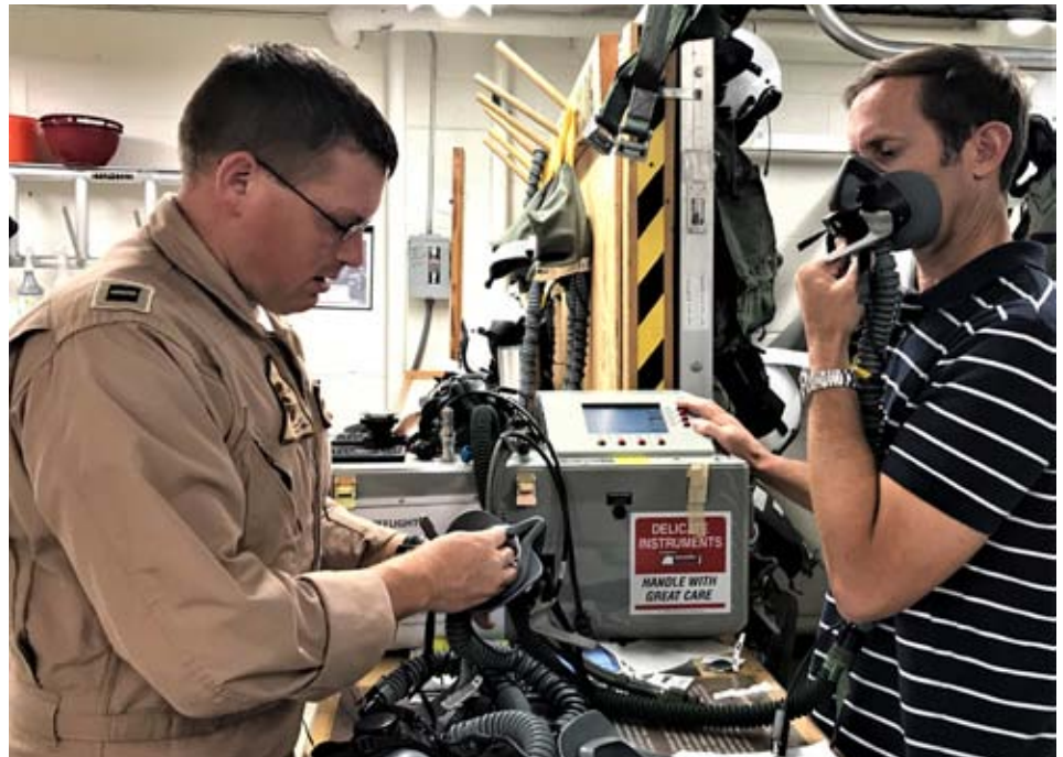
PENSACOLA, Florida Lt. Daniel Logsdon CTW-6 AMSO and Jeff Henderson NAVAIR Aircrew Oxygen Systems performing a one-time inspection on the MBU-23 mask. Photo by Jackie Hillies.
