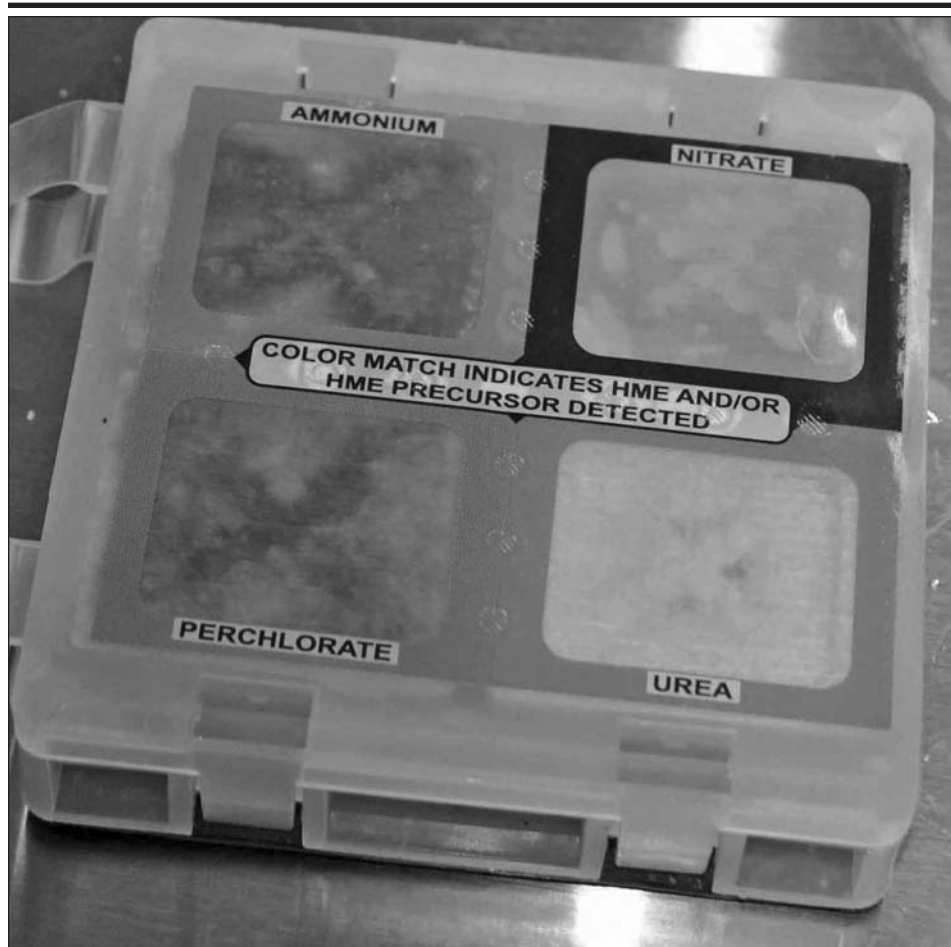
Chemical Reconnaissance and Explosives Screening Set or CRESS. The kit can screen for dangerous fuel and oxidizer chemicals such as perchlorate, urea, nitrate, and ammonium. U.S. ARMY PHOTO BY RACHEL SELBY
