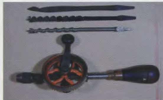
Hart's hand drill and bits. Most of the tools in the collection are in good, working order and could still be used to build items. (Photo by Mike Taylor)
