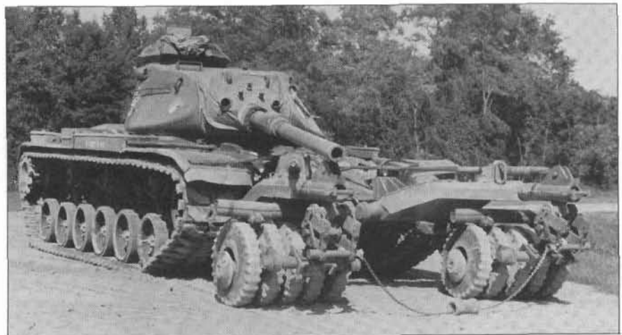
The track-width mine roller was issued to armor units in Europe last year. The roller was reverse engineered from the Soviet PT55/KMT5.
