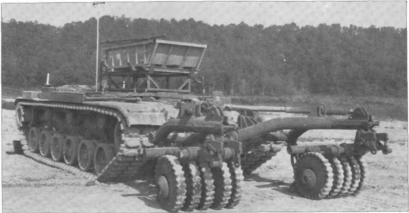
The Robotic Obstacle Breaching Assault Tank (ROBAT) is slated for heavy division engineers. ROBAT detects, neutralizes and marks lanes by remote or manual control.
