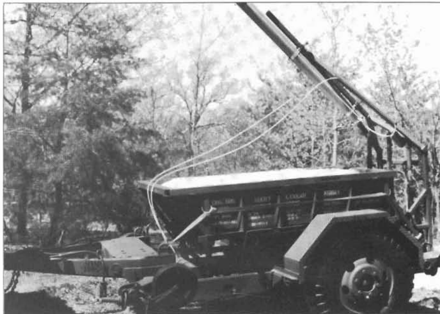
This USMC Mine Clearing Line Charge (MICLEC) is being evaluated as a countermine option for light units.
