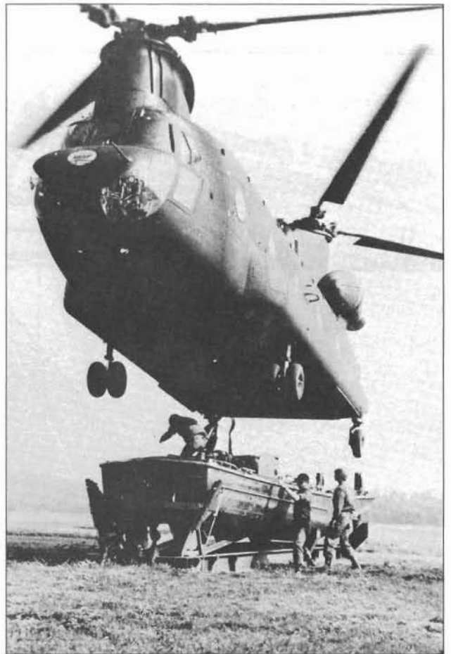
Helicopter (above) delivers a Bridge Erection Boat. (Photo by SFC Dennis O. Lindsey.)
