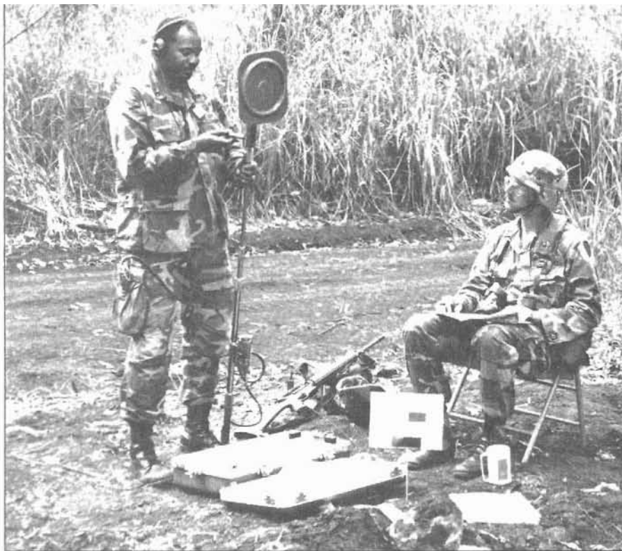
The Expert Sapper Test emphasized testing and training. Each candidate was thoroughly debriefed on their performance for each activity. Here SSG Chapman assesses SSG Lee's knowledge of the AN-PSS 11 mine detector.
