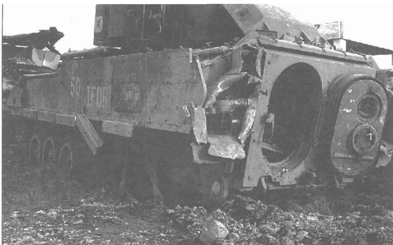
The hazards of operations in a mined environment—an M2 Bradley after striking a TMA-3 antitank mine.
