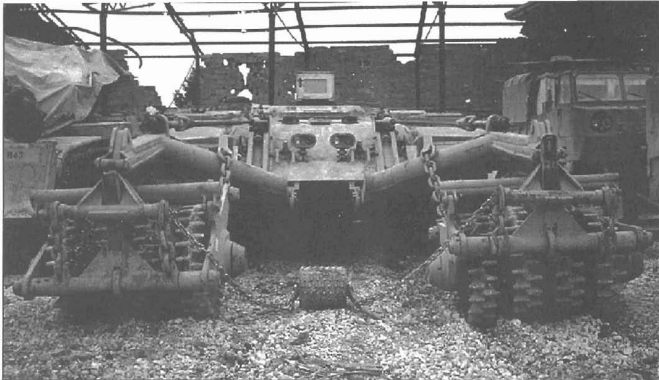
M60 Panther countermine vehicle with track-width mine rollers and improved dogbone assembly.
