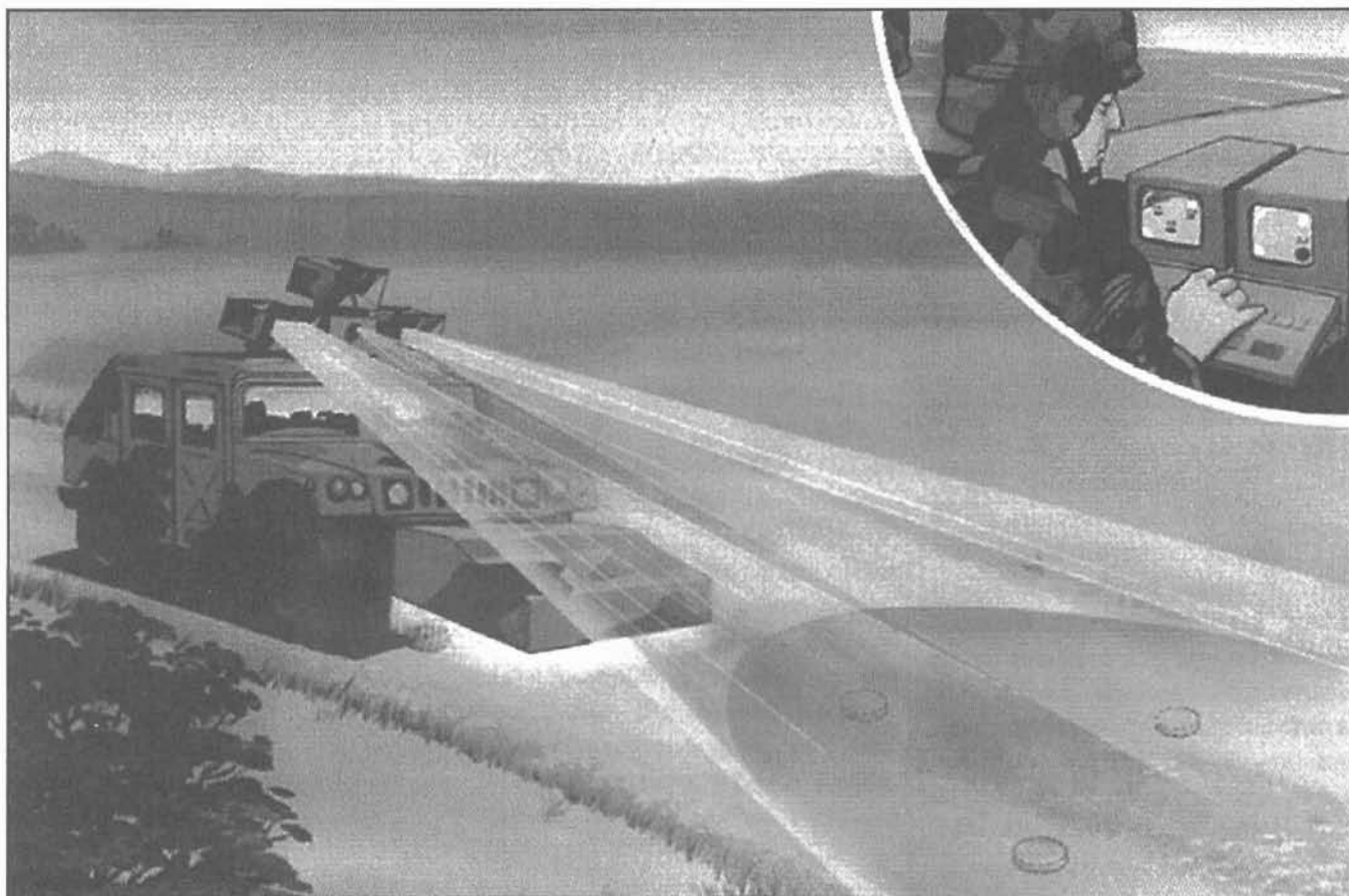
GSTAMIDS is a multisensor vehicle-mounted mine detector. It is in concept exploration with development scheduled to begin in FY98. This concept drawing shows GSTAMIDS mounted on a teleoperated HMMWV. The actual system will be different.
