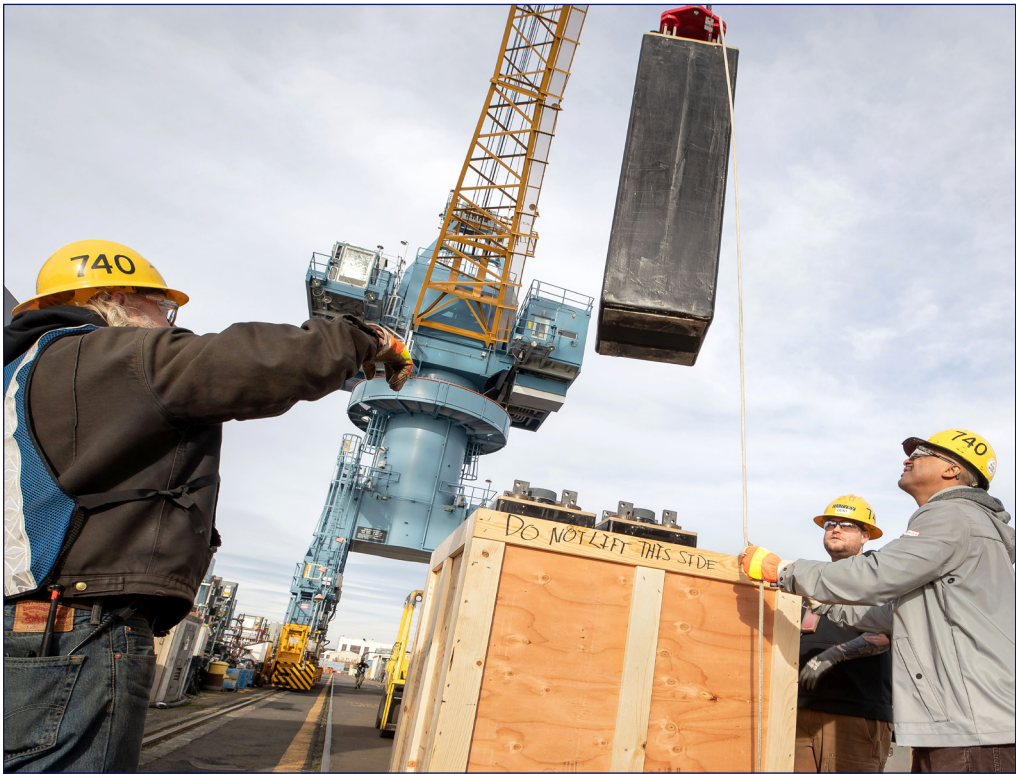
Bruce Robertson left, Steven Dent and Senteil Andrews, Code 740 riggers, land the battery cell removed from USS Bremerton (SSN 698). (PSNS & IMF photo by Scott Hansen)
