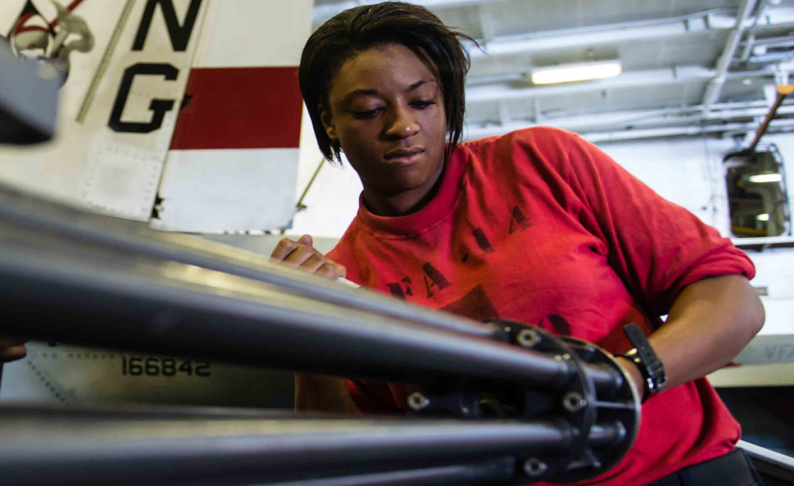
↑ Airman Jasmine Yelberton performs maintenance on an M61A2 20mm machine gun for an F/A-18E Super Hornet assigned to the Top Hatters of Strike Fighter Squadron (VFA) 14. (Photo by Petty Officer 3rd Class Andre T. Richard)
