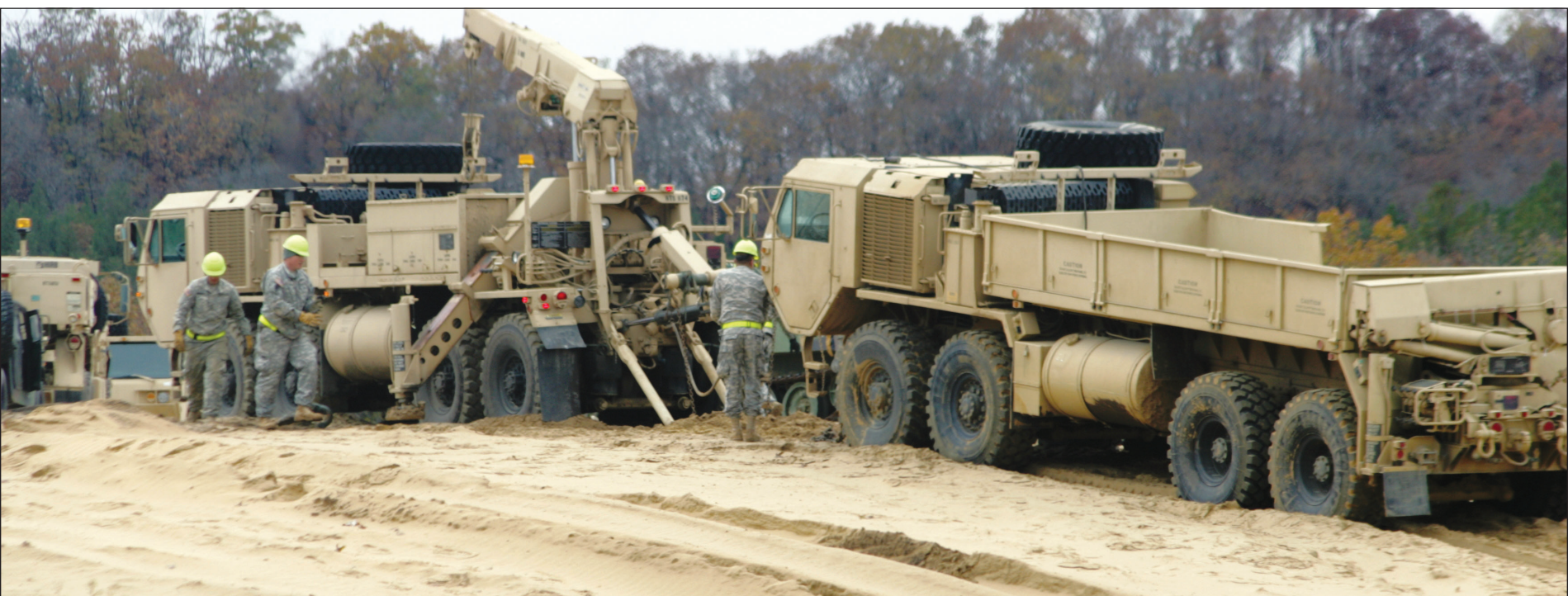
Students return equipment to an M984A4 Recovery Truck (Wrecker) after recovering a tactical vehicle that was mired in sand at the Vehicle Recovery Site.
