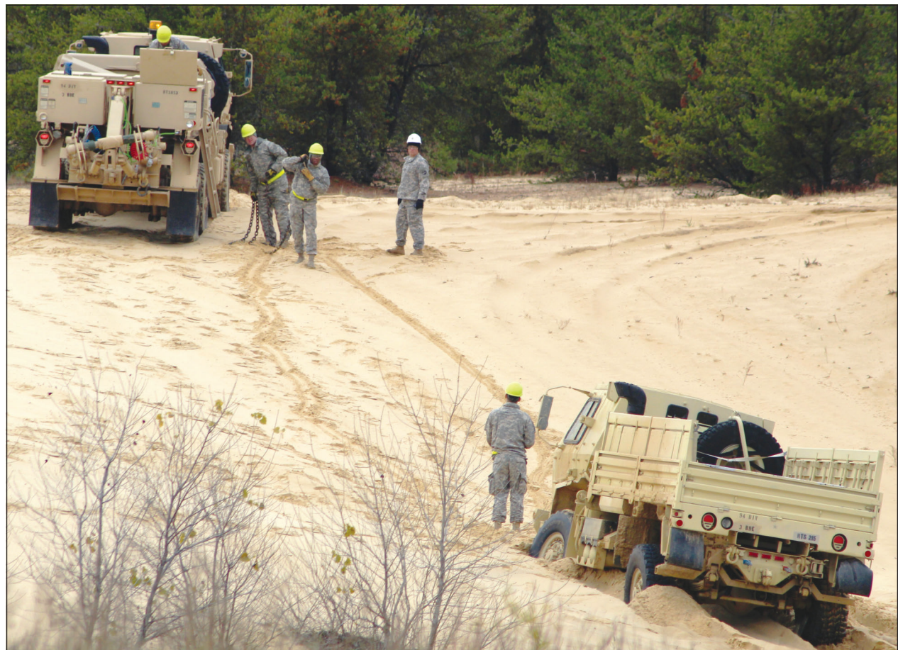
Students in the Regional Training Site-Maintenance Wheeled-Vehicle Recovery Operations Course practice vehicle recovery at the Fort McCoy Vehicle Recovery Site on Fort McCoy's South Post.
