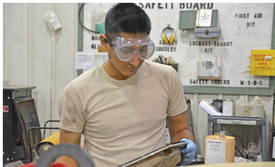
Sgt. 1st Class Stephanie Widemond Spc. Jhon Cubas, 2-349th LSB mechanic, inspects a transmission pan gasket prior to reinstalling it as part of repairs done to keep a vehicle mission ready.
