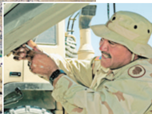
Spc. David S. Ige of Hilo bleeds the fluid lines of a grader before it goes out to work on the Tarin Kowt Road.
