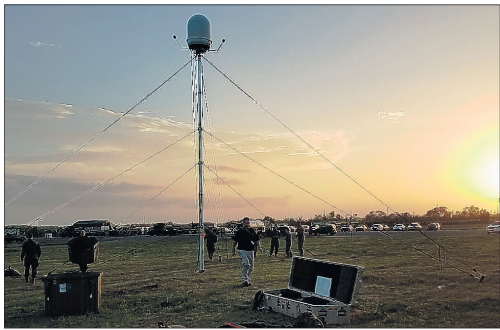
The Meteorological Mobile Facility (Replacement) Next Generation (METMF(R) NEXGEN) weather radar stands fully assembled at sunset.
