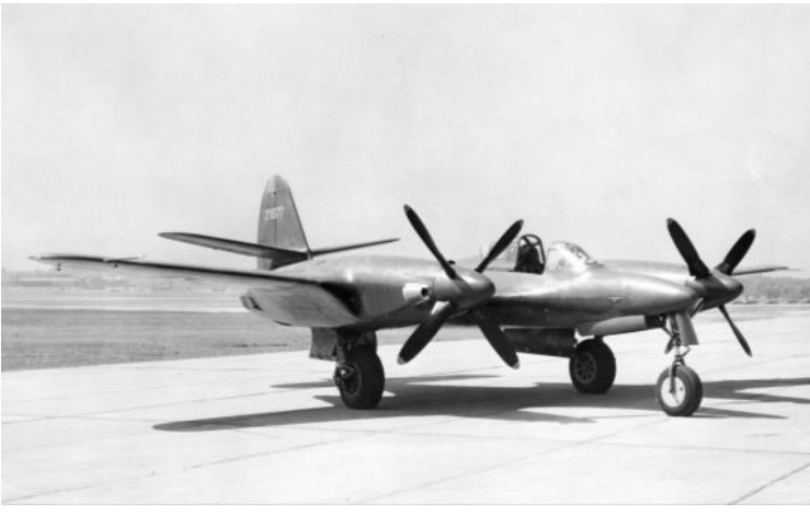
The McDonnell XP-67 Moonbat was first aircraft they produced. Though unsuccessful, it led the way to the FH-1 Phantom and eventually F2H Banshee jets. (U.S. Navy photo)
