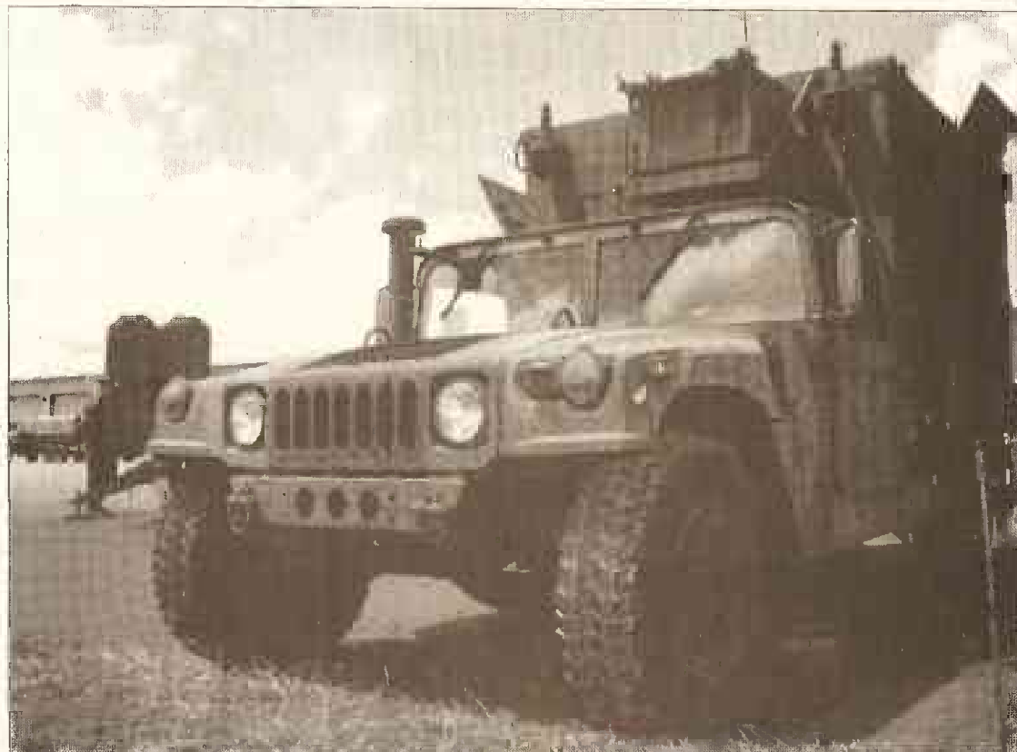
LCpl. Steven Williams The AN-TMQ 41 Meteorological Measuring Set is a high-tech combat weather system used to decipher atmospheric conditions in a field environment.
