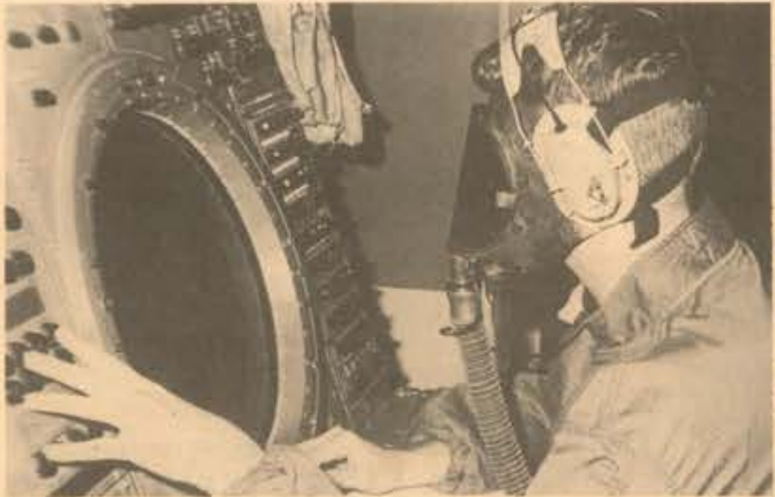
EYE ON THE SKY — An air traffic controller from Marine Air Control Squadron-2, carefully monitors his radar for incoming traffic. The controllers use the M-24 gas mask to communicate with aircraft. The mask differs from the M-17, in that it allows for the use of headsets and microphones.
