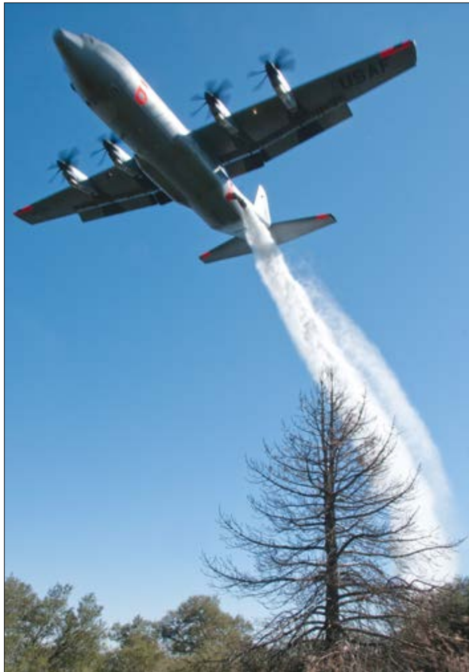
A C-130J airtanker from the 146th Airlift Wing, equipped with the Modular Airborne Fire Fighting System II, drops water during annual firefighting training with U.S. Forest Service aviators near Channel Islands Air National Guard Base in Port Hueneme, Calif.
