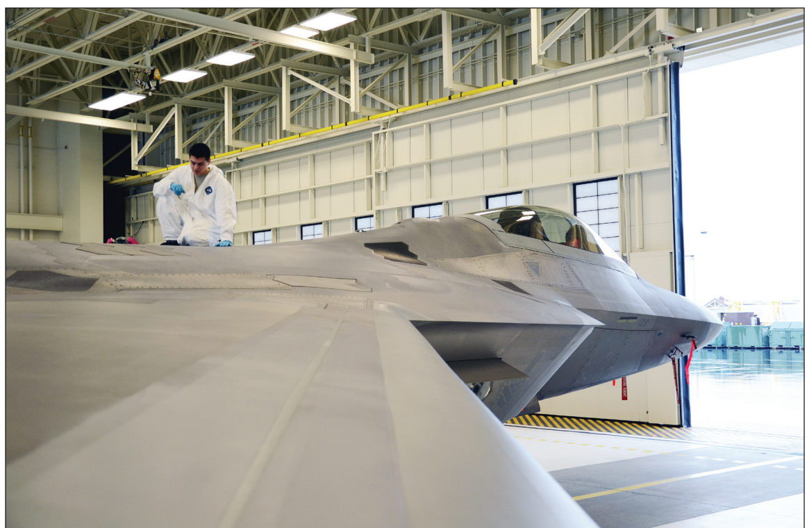
Airman 1st Class Emmanuel Marioni, 3rd Maintenance Squadron, inspects the skin of a 3rd Wing F-22 Raptor Sept. 28. Marioni is a low observable technician with the 3rd Maintenance Squadron. (U.S. Air Force photo/Senior Airman Joan King)
